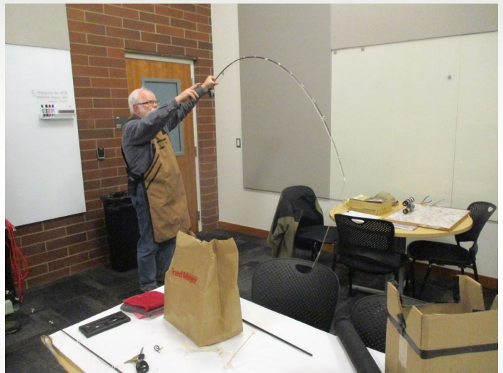
Richard checking the static load guide position to ensure proper guide spacing and placement.
